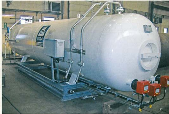
Fig. 1: A high pressure CO 2 tank
